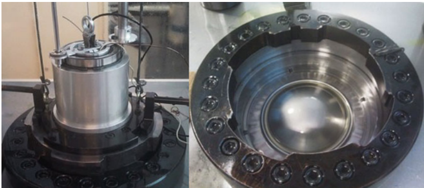
Fig. 7 Experimental system used for biaxial hydraulic bulge test
