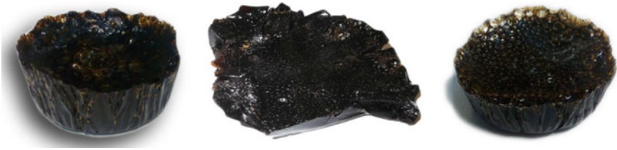
Fig. 9 Samples of coffee-PLA mixtures. The samples presented here represent the experimental mixture between PLA and coffee powder
