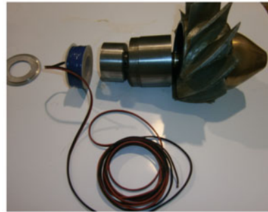
Fig. 3 Sketch of the MRB system ( left ) and picture with mounted pieces ( right )
