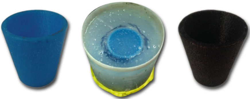
Fig. 10 3D printed part in PLA ( left ), Silicone mould ( centre ) and casted part ( right )
