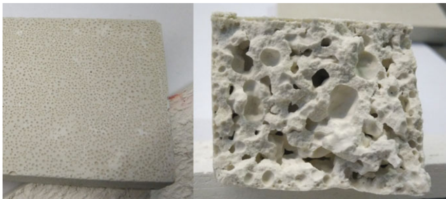
Fig. 10 Samples with abundant pores
