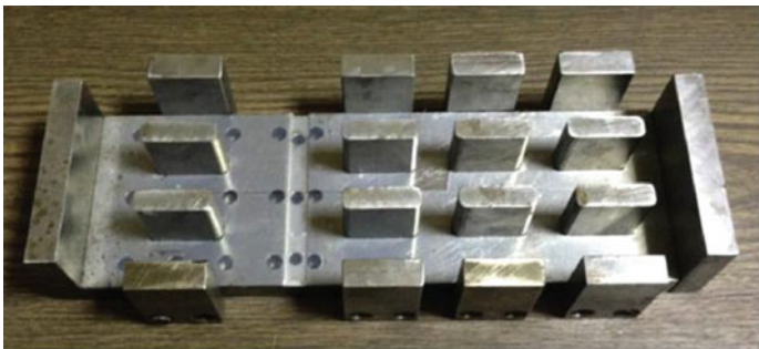
Fig. 2 The mold used to prepare the samples
