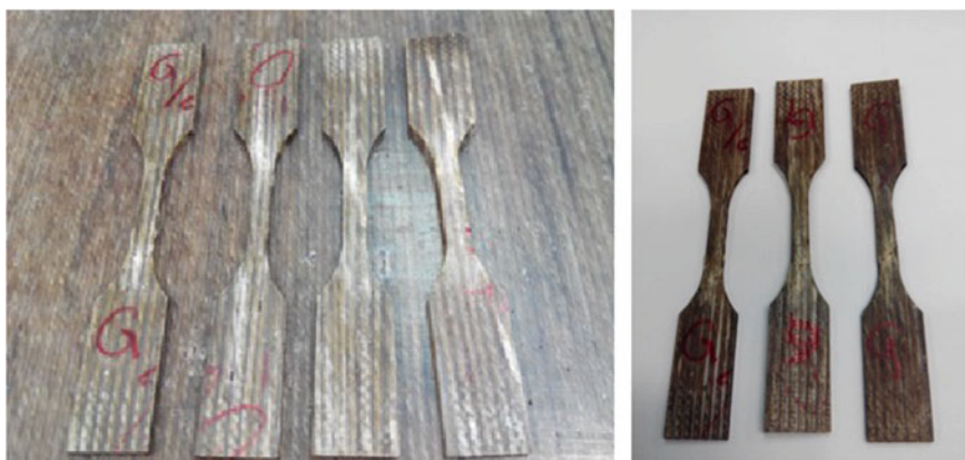
Fig. 2 Composite specimens for tensile tests
