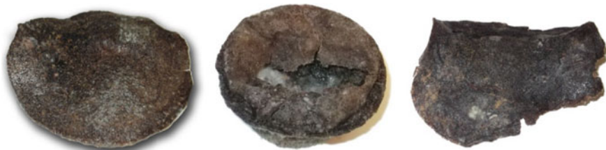
Fig. 6 Degradation of the mixtures with starch. After one month, all results that used starch showed humidity problems with the presence of mold
