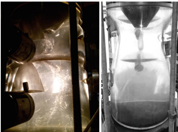
Fig. 7 Visualization of the cavitating flow from the test rig at: 1020 rpm (right) and 690 rpm(left)
