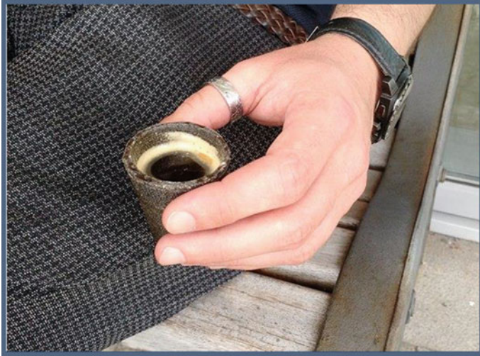
Fig. 12 Experimenting the material in contact with hot beverage (coffee). It is also noticeable that the heat from the hot coffee does not pass to the exterior
