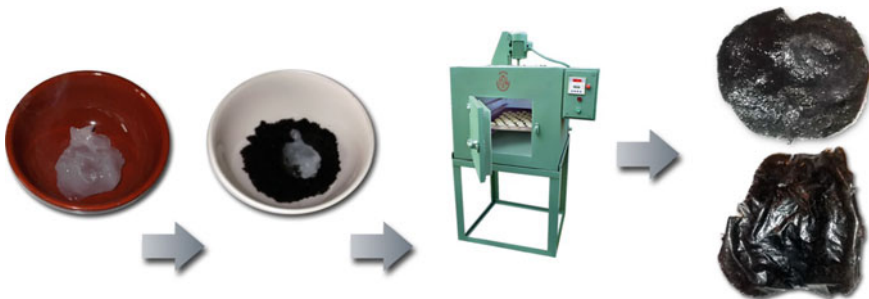
Fig. 5 Mixtures with starch. Bowls with potato starch and cold water mixture and addition of coffee powder ( left ). Industrial oven ( centre ). Results after heating ( right )
