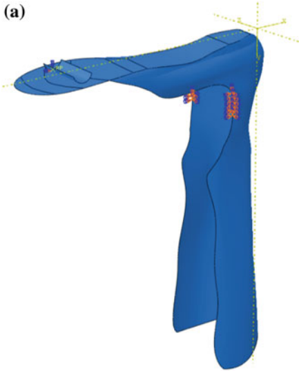
Fig. 3 Finite element model of the orthosis (a) and mesh (b)
