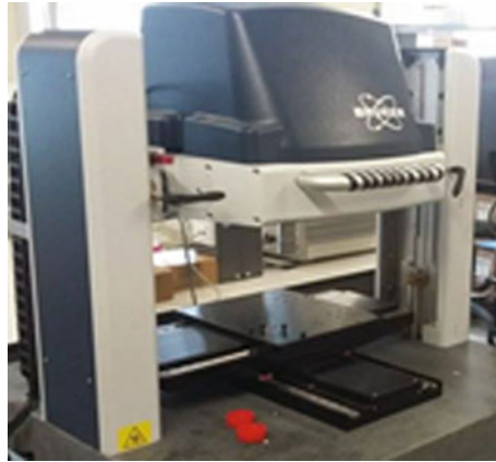
Fig. 4 Bruker NPFLEX equipment utilized to measure the roughness
