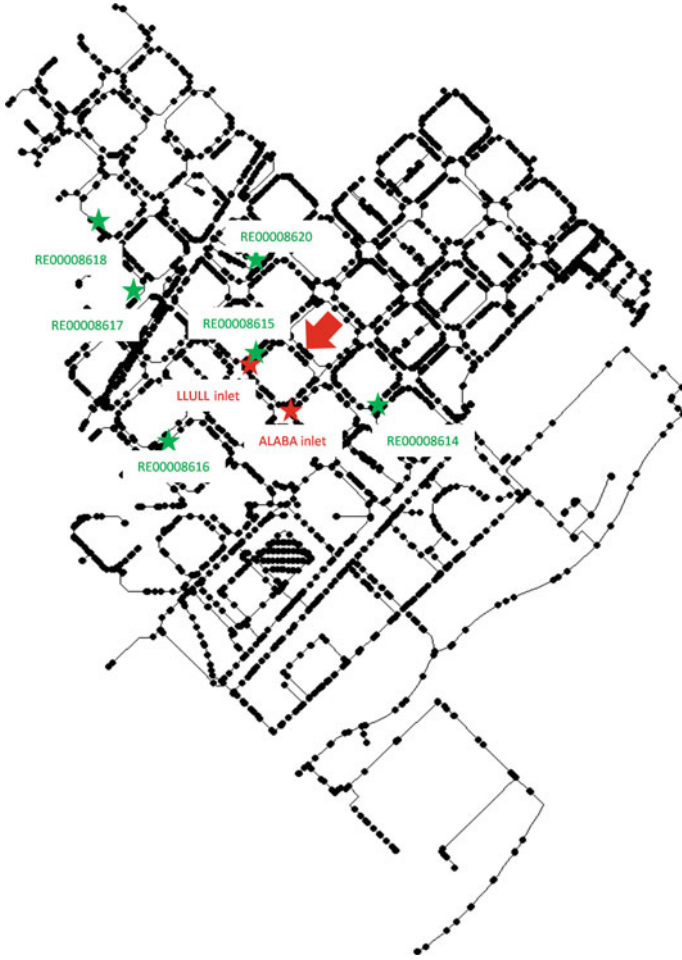
Fig. 7.2 The water network of Nova Icària district metered area (DMA) (EPANET model) highlighting inner pressure sensors ( green stars ), DMA inlets ( red stars ) and the exact location of the leak ( red arrow ) that was intentionally introduced to test the method
