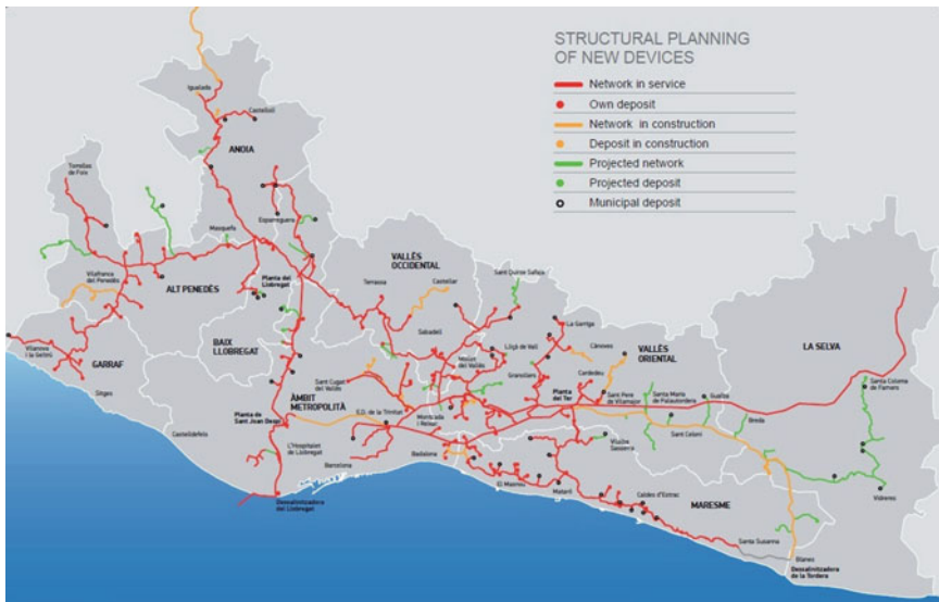
Fig. 10.6 ATLLs Catalonia regional water network
