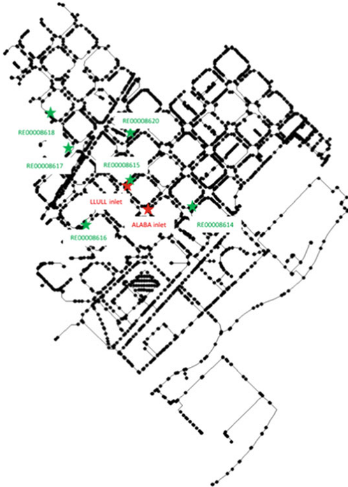
Fig. 2.8 Nova Içària DMA. In red, the two inflows, (flow and pressure sensors) and in green, the inner pressure sensors
