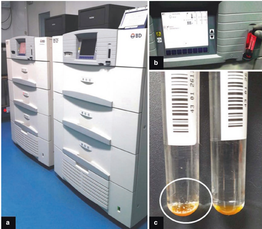
Fig. 26.3 Isolation of Mycobacterium tuberculosis by semi-automated liquid culture system. (a) BACTEC MGIT 960 machine (Beckton, Dickson, Sparks, Md.); (b)
