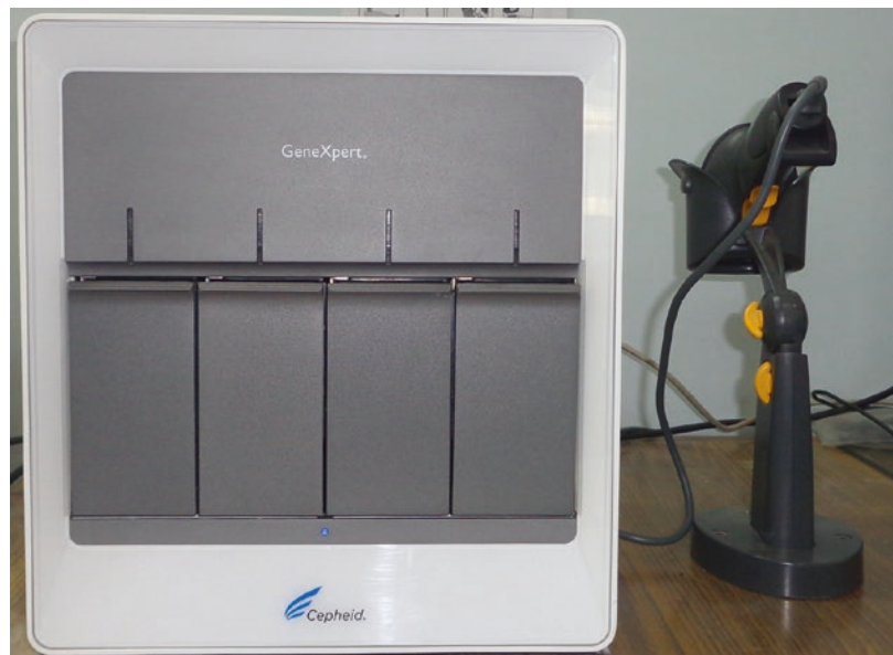
Fig. 26.4 Xpert MTB/RIF machine, a model for processing of four samples simultaneously
