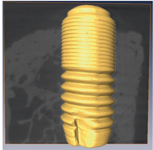
Fig. 3.1 Micro-CT imaging of cancellous and cortical bone healing around an oral implant. Image shows both the intimate contact in the transcortical region and the cancellous bone adaptation to the mid-body of the implant
