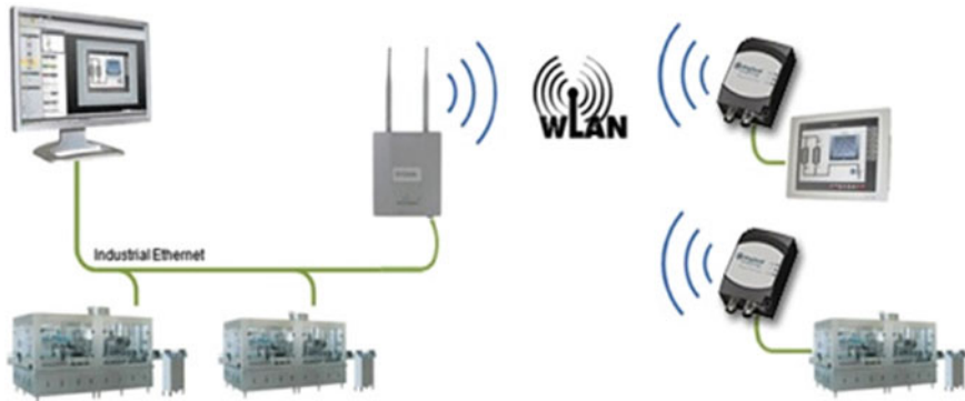
Fig. 2 An example of industrial IoT communication architecture
