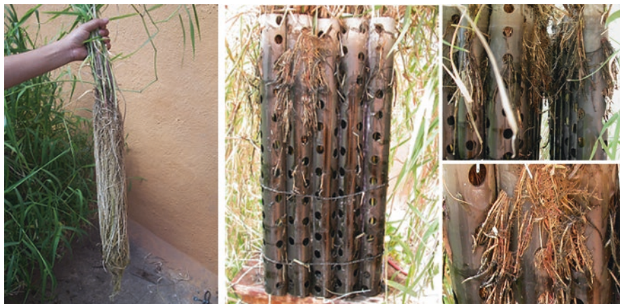
Fig. 1.5 Ideal root system growth of Phragmites sp. in the Bio-rack at steady-state condition
