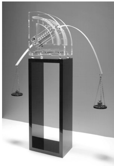
Fig. 4.14 The elastica arm scale. Image courtesy of Davide Bigoni.
