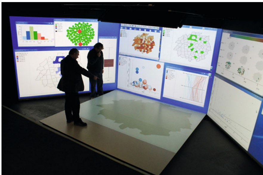
Fig. 11.1 GeoDa in the Virtual Reality CAVE displaying multiple dynamically linked panels of analyses linked via brushing and linking to each other and to the map display on the floor
