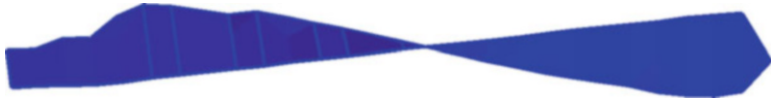
Fig. 21.25 Blade displacement mode shape first torsional mode—identification using roving hammer impact test with strain gauge as reference
