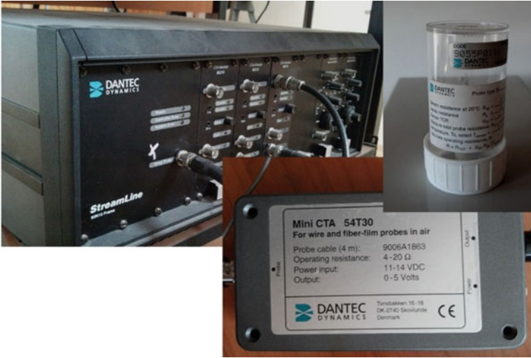
Fig. 13.15 MiniCTA 54T30 DANTEC, StreamLine 90N10 Frame, and CTA probe DANTEC
