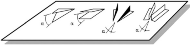
Fig. 1.3 Different types of vortex generators. From left to right: delta wing, rectangular wing, delta winglets and rectangular winglets (Chu et al. 2009)
