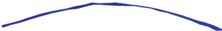
Fig. 21.23 Blade displacement mode shape first bending mode—identification using roving hammer impact test with strain gauge as reference
