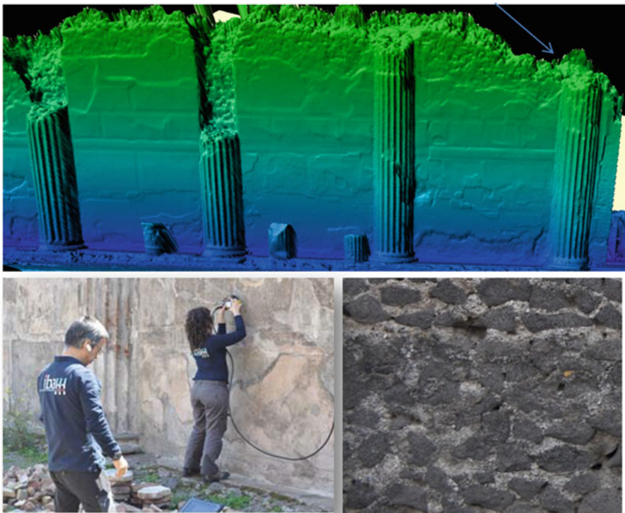
Fig. 29.2 Top : Digital model of southern wall of the Basilica investigated by GPR and seismic tomography. The wall is interrupted by plastered fluted semicolumns built with bricks. Bottom left : GPR data acquisition. Bottom right : Detail of the masonry composed of irregular stone elements of Peperino
