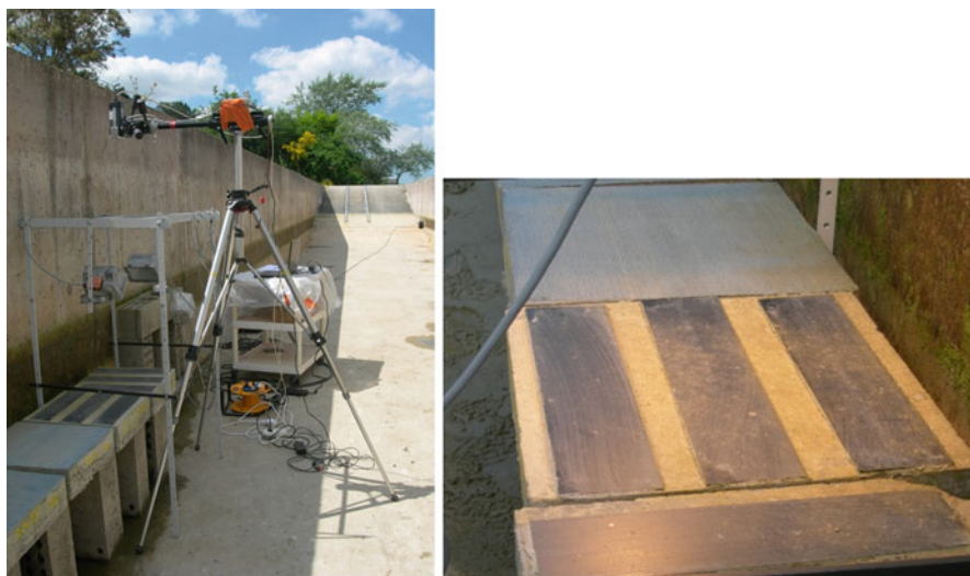
Fig. 11.13 View of outdoor test site with an active infrared (IR) test bench over the specimen ( left panel ). Detailed view of the specimen surface during thermal solicitation ( right panel )
