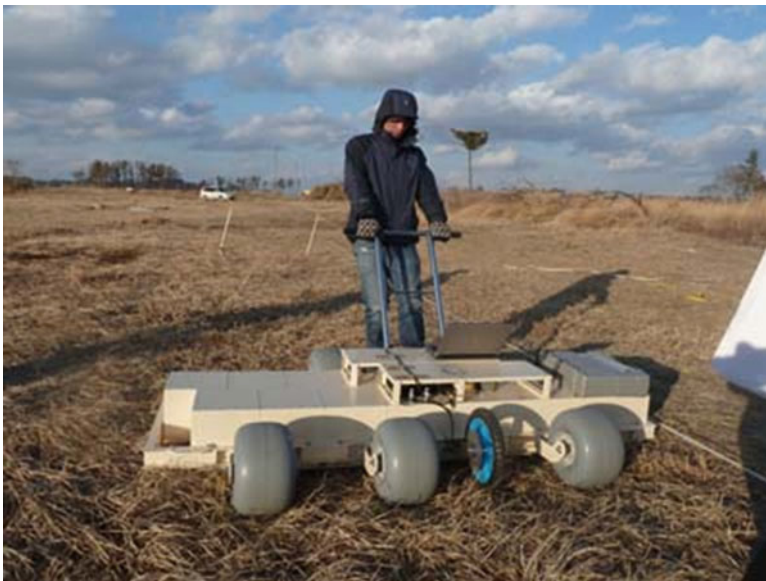
Fig. 9.7 The array GPR system “Yakumo,” developed by Tohoku University, is equipped with eight transmitting and eight receiving antennas (Nobiru Site, Japan)
