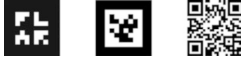
Fig. 20.1 From left to right . First two pictures: Examples of synthetic images used as fiducial markers for AR applications. They are very similar to 2D QR codes, shown in the third picture, that can be used as target images as well
