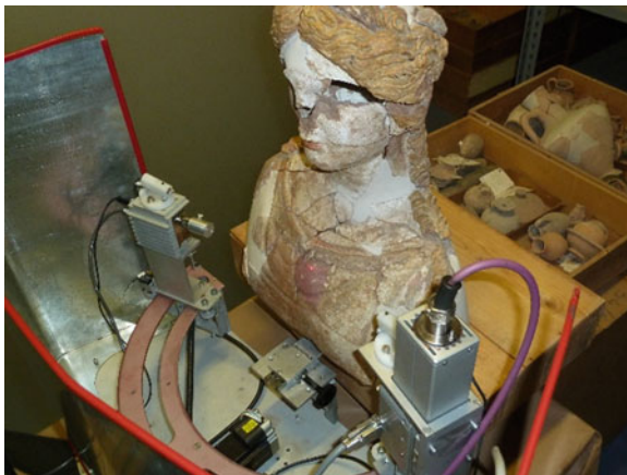
Fig. 15.2 The portable X-ray diffraction (XRD) spectrometer during the analysis of a Hellenistic sculpture at the Paolo Orsi Archeological Museum in Syracuse (Italy)
