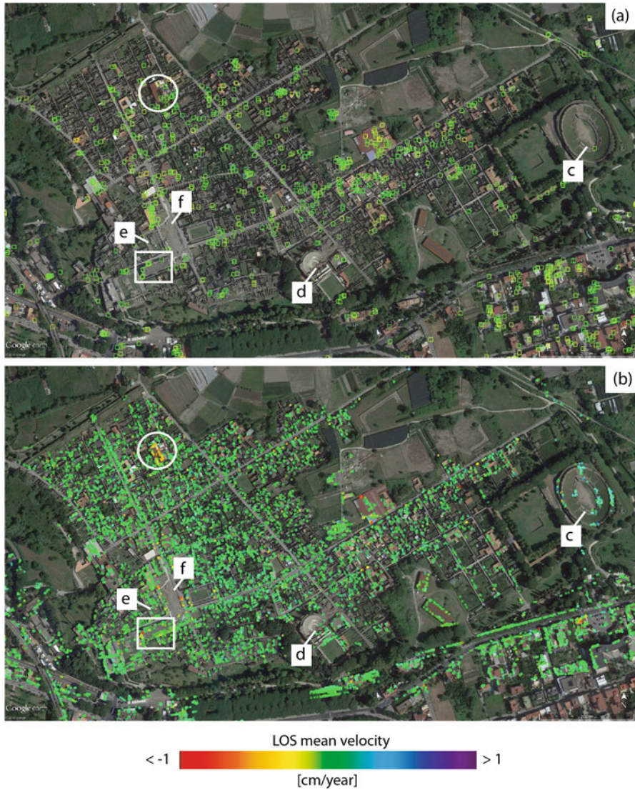
Fig. 6.4 Comparison between the ERS/ENVISAT and the CSK SBAS-DInSAR results relevant to the selected area shown in Fig. 6.3. (a) Zoomed view of the full-resolution SBAS-DInSAR results achieved through the 1993–2010 ERS-1/2 and ENVISAT SAR data archive. (b) Zoomed view of the full-resolution SBAS-DInSAR results achieved through the 2009–2015 CSK SAR data archive. Some well-known historical and archaeological monuments, such as the Major Amphitheatre (label c ), the Big Theatre (label d ), the Temple of Apollo (label e ) and the Roman Forum (label f ) are also highlighted. The white circles indicate the position of the historical building (the “House of Vettii”) investigated in Fig. 6.5, whereas the white rectangles show the location of the “Basilica,” analyzed in Fig. 6.6
