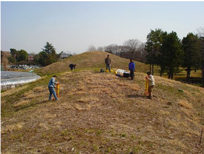
Fig. 27.2 Three-dimensional ground-penetrating radar (3DGPR) survey on Okunoyama-kofun tumulus at the Sakitama-kofun tumulus site, Japan
