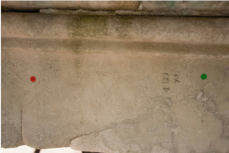
Fig. 12.13 Waveforms along a profile at the surface of the Carrara marble ( above ). Red crosses mark the arrival of the Rayleigh wave. The average Rayleigh wave velocity is given in the boxes on the above top . Location of the profile ( below ). The position of the source is indicated by the red point . The end of the profile is marked by the green dot (Photograph published with permission by Stiftung Preussische Schlösser und Gärten Berlin-Brandenburg)
