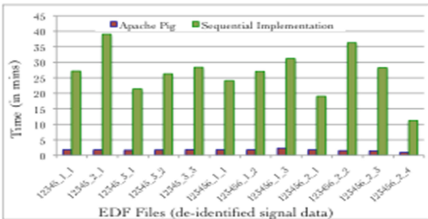
Fig. 2. A comparative evaluation of processing time for 12 EDF files with different sizes using Apache Pig and sequential evaluation demonstrates the significant improvement in data processing time.
