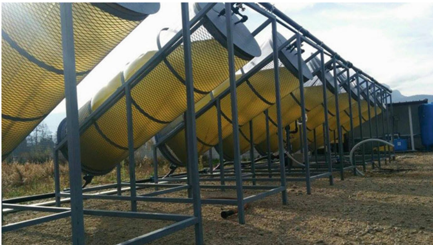
Fig. 4 Bubble columns made of polypropylene foils molded in cylindric shape. Columns are supported by steel scaffolds and inclined toward sunlight
