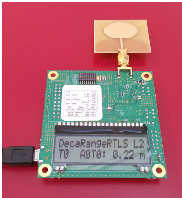
Fig. 7.8 Decawave UWB module for ranging with decimetre level accuracy and tens of metres reach
