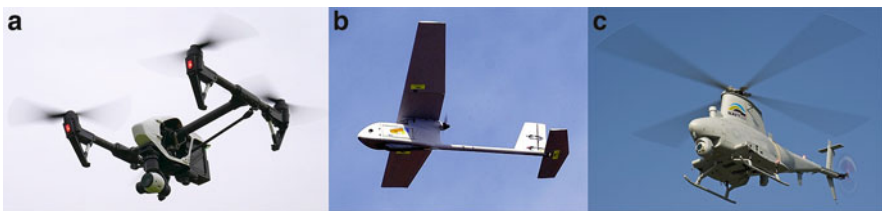
Fig. 15.1 Types of UAV. From left to right : (a) Quadcopter, (b) Fixed-wing and (c) Biofuel copter
