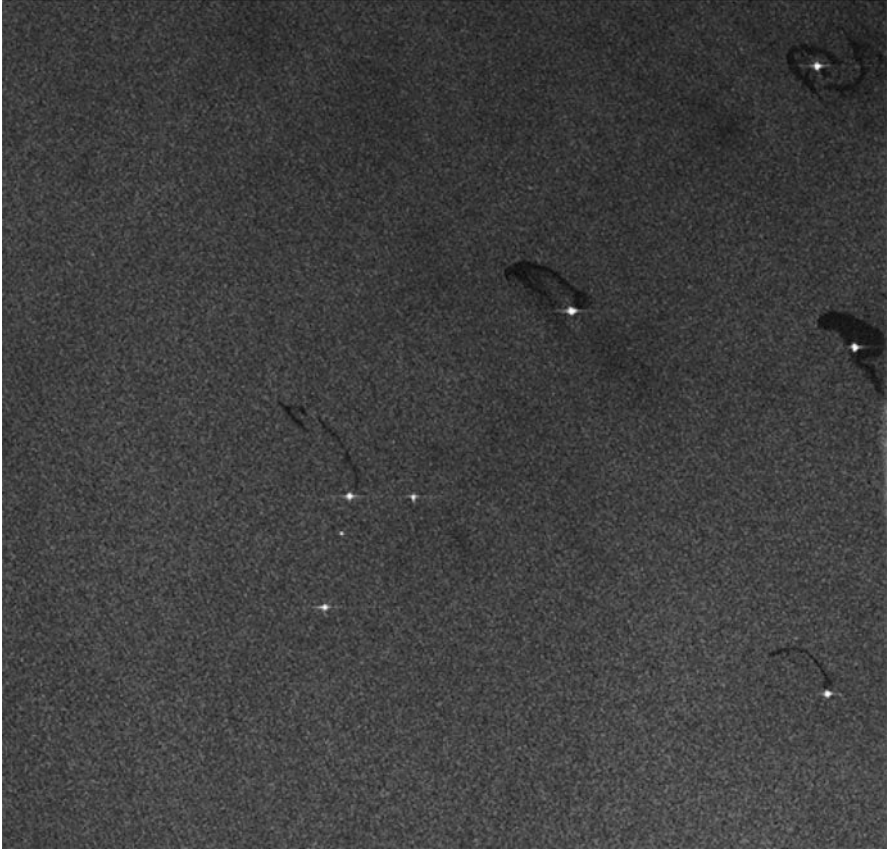
Fig. 11.6 Example of water contamination by oil platforms off the coast of Norway. Radar image is taken from Sentinel-1a, 2014. Copy right: European Space Agency. Image is reproduced with the permission of European Space Agency
