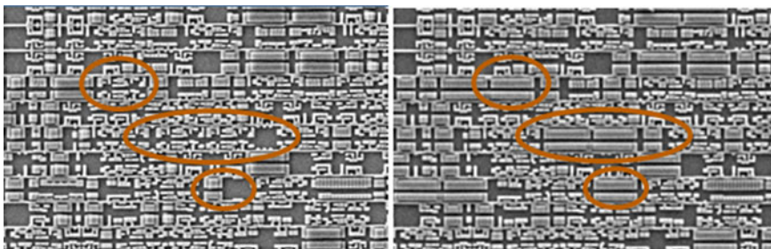
Fig. 7.19 Left Infected circuit HT area, right genuine circuit identical area
