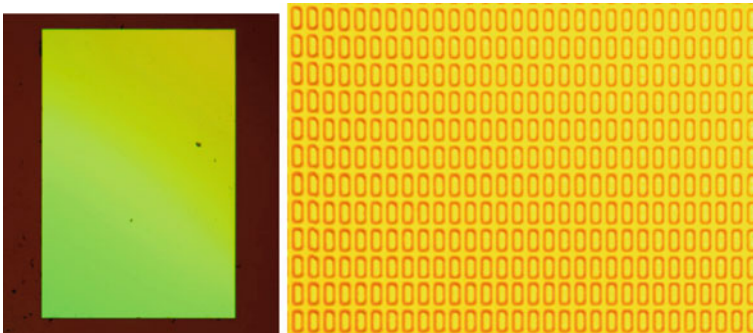
Fig. 7.4 Frontside and backside visible light acquisitions of an integrated circuit
