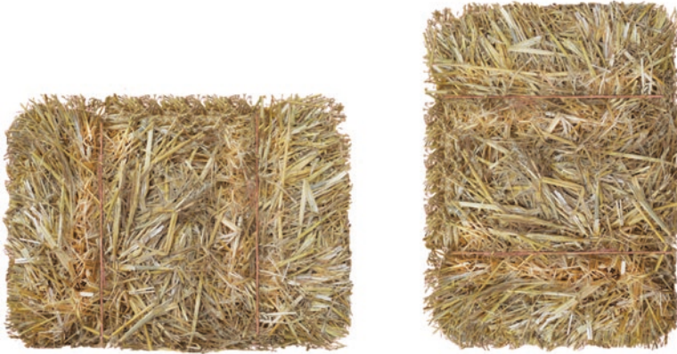
Fig. 20.4 The bale on the left is as it emerges from a baler. The bale on the right as installed in the ModCell Core Passiv wall so the y coordinate is vertical
