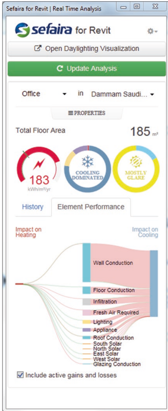
Fig. 10.7 Energy consumption analysis on the case study residential building in the city of Dammam KSA—with the use of insulation materials on external walls
