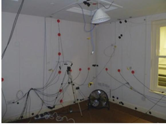
Fig. 9.1 Photograph of bedroom 1 in the test house showing HFPs (red discs) on the thermal elements
