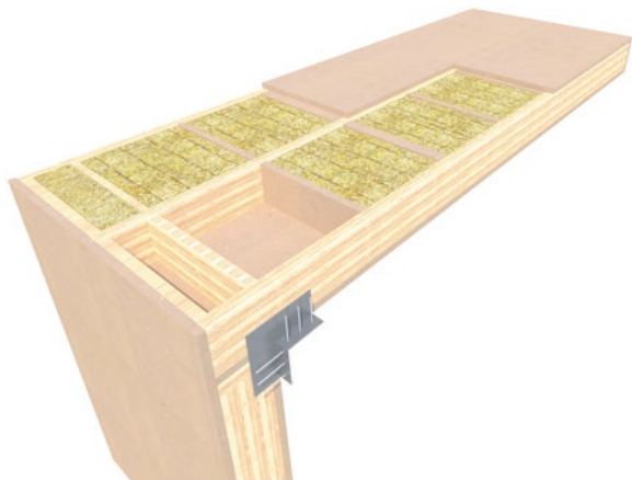
Fig. 20.12 Perspective of roof cassette module
