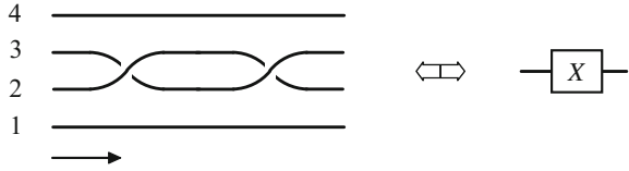
Fig. 3 Braiding diagram for the Pauli X gate and its quantum computation symbol
