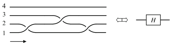
Fig. 4 Hadamard gate implemented by braiding and its quantum computation symbol
