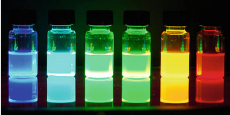
Fig. 17.18 Alloyed quantum dot emits light of different wavelengths by tuning the composition [84]
