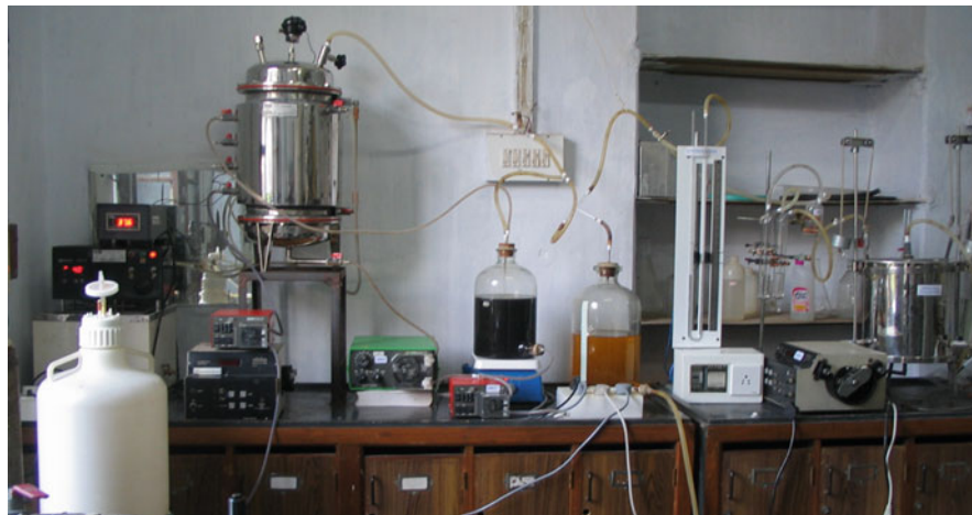
Fig. 16.3 Continuous biohydrogen production using cane molasses as substrate in 20 L packed bed reactor
