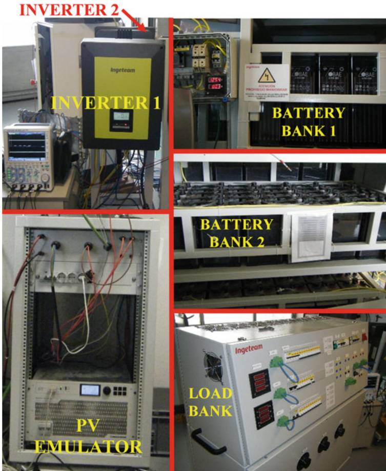
Fig. 21 Experimental setup, showing the PV emulator, battery and load banks [7]
