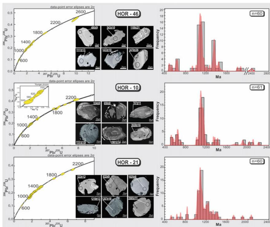
**Fig. 9** U-Pb (LA-ICP-MS) concordia diagrams, frequency histograms and some of the electronic microscope (SEM) images of the studied zircon grains from samples Hor 46, Hor 10 and Hor 21. The location of the spots and obtained ages by LA-ICP-MS are in Ma. See Tables 3, 4 and 5 (supplementary material)
