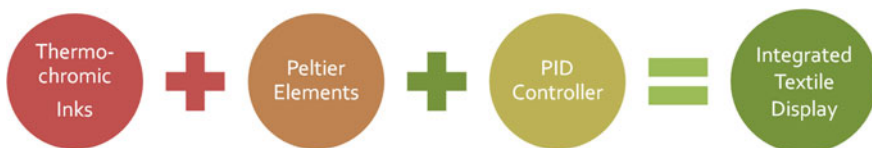
Fig. 5.1 Overview of the technological components used to implement non-light-emissive animatable textile displays
