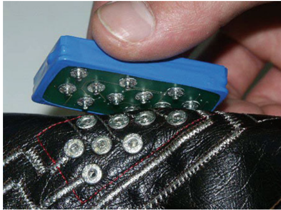
Fig. 9.2 Snap fasteners with female part on leather and male part on a PCB. Image courtesy of Linz et al. at Fraunhofer Institute [20]
