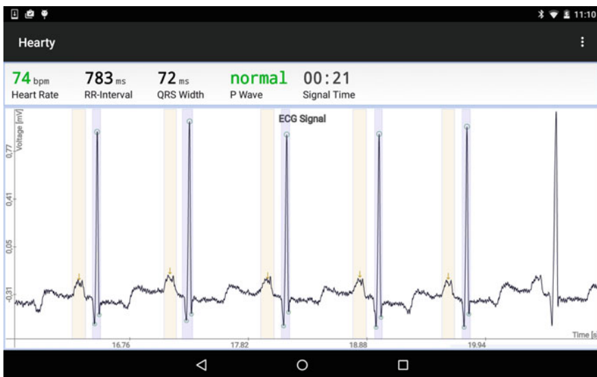
Fig. 16.3 Screenshot of the Hearty application [13] running on a typical off-the-shelf Android tablet and processing an ECG record in quasi real time. In the upper area of the interface, typical ECG-related statistics are displayed (from left to right heart rate in beats per minute, RR interval in ms, QRS width in ms, the classification of the P wave, and the runtime of the current signal). In the lower area of the interface, the raw signal is displayed continuously. As soon as the processing algorithm detects an R-peak, the QRS width is extracted and the QRS complex colored in light blue . After detecting the P wave, it is colored in light brown with an arrow indicating the assumed P-peak position
