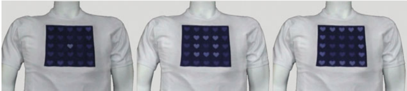
(b) Tshirt with a pixelated wearable display.
