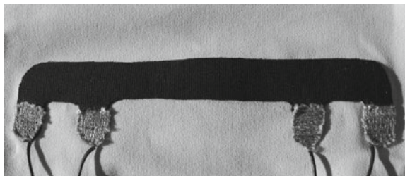
Fig. 4.3 Single-layer KPF sample attached to a lycra® substrate
