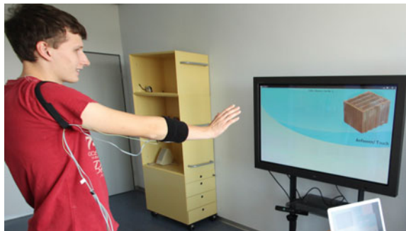
Fig. 6.7 A user receives haptic feedback when approaching an object shown on the screen
