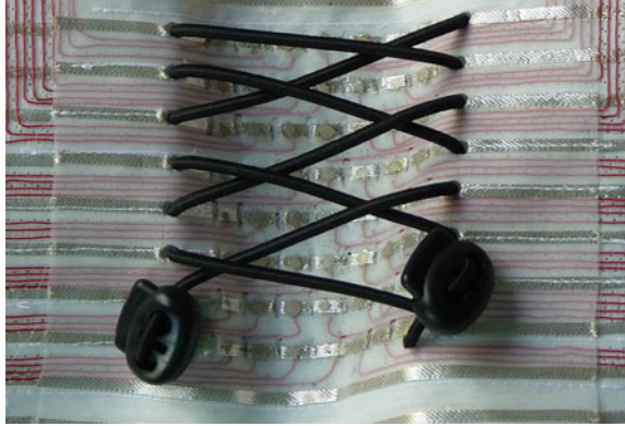
Fig. 9.10 Pocket version with elastic cords. This version allows the reader to see the conductive pads inside, while the elastic cords generate the pressure between textile and device
