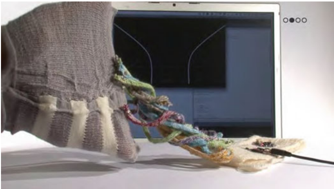
Fig. 11.15 Shape sensor: three conductive rows on the knitted tube act as analog sensors detecting the shape of the stretched tube
