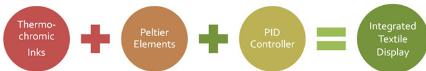
Fig. 5.1 Overview of the technological components used to implement non-light-emissive animatable textile displays
