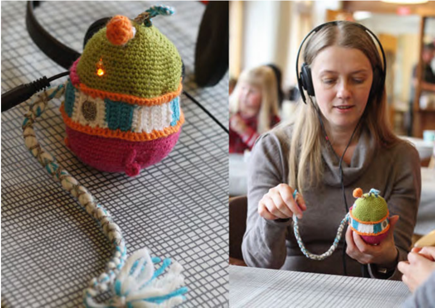
Fig. 11.3 The Soft Radio: a crocheted radio that uses textile interactions of wrapping and twisting for operating the radio. Video available at http://narrativize.net/softradio/
