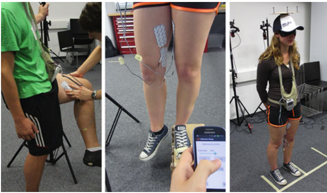
Fig. 6.11 Placing the electrodes on the musculus sartorius ( left ) and measuring the angle of deflection corresponding to EMS intensity ( right )
