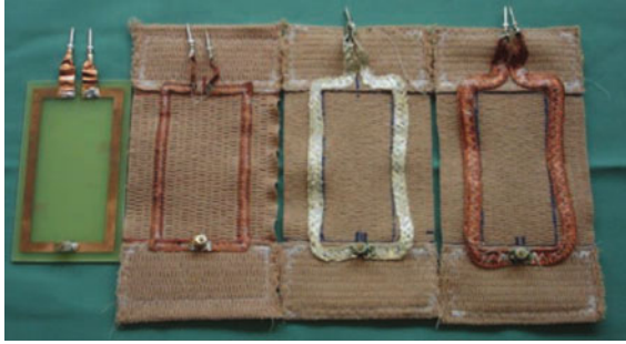
Fig. 7.3 Reference coil on a circuit board and three stretchable coils on elastic fabric. The elastic fabric is 91% cotton and 9% polyamide. The conductors are, from left to right , copper braids of 5 mm, 7 mm with silver coating and 9 mm. © 2011, John Wiley and Sons. Reprinted with permission from [17]
