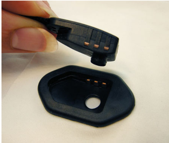
Fig. 9.3 Plug connector with female part integrated into textile. Image courtesy of Ohmatex [24]
