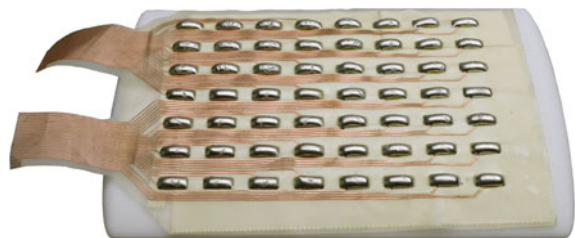
Fig. 9.9 3D-printed casing with attached flexible print with solder bumps. The casing is 100 mm long and 75 mm wide. The curvature is elliptic with 16 mm minor axis
