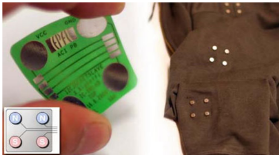
Fig. 9.4 Magnetic connectors for I2C printed circuit board. © 2010 IEEE. Reprinted with permission from [30]
