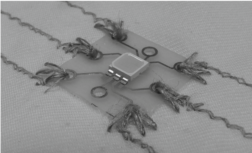
Fig. 2.14 SMD electrically and mechanically connected with conductive thread (Image courtesy of ITV Denksdorf)
