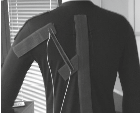
Fig. 4.10 Single-layer strain sensor is positioned in the scapular area in order to detect scapular elevations and abductions
