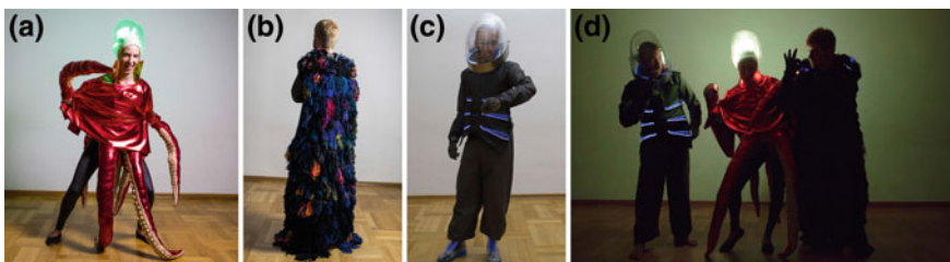
Fig. 13.7 a The Octopus Sea Creature can move two tentacles at its front through motorized skeletons and has a glowing brain for expressing its moods. b Captain Nemo has a living robe which can glow in the dark and vibrates if someone comes closer to the integrated distance sensor. c The Diving Suit has a fin-like pattern that glows blue or white according to sea or land mode and wears an oxygen tank which can be controlled via a display on the suits glove. d All costumes in the dark. Photographs by Marko Schmidt/Jena. Image courtesy of HCI Group (c), Bauhaus-Universitaet Weimar
