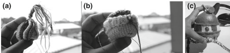
Fig. 11.12 Examples of the form iterations for enabling textile contacts with wrapping: a A central sphere with vertical flaps forming overlapping layers. A furry chord could be wrapped so that it goes between the flaps. b A sphere with conductive parts along its equator and a “tail” that could be wrapped around it. The chord would touch the conductive parts in different orders depending on the direction of the wrapping. c The resulting form of the Soft Radio
