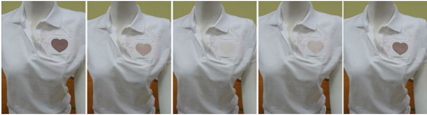
(a) Tshirt with an animated heart using a single wearable animated pixel.
