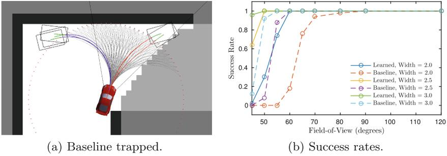
**Fig. 4.** (a) Baseline planner trapped, steering away from the goal, due to insufficient observed free space to the right. The only feasible actions, that are both collision-free and have a feasible emergency-stop action, are blue. See main text for discussion. (b) Success rates in reaching the goal as a function of hallway width and field-of-view, for our method and the baseline planner.
