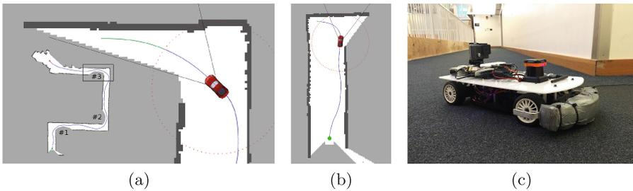
**Fig. 7.** (a) Experimental trajectory of our planner through a hallway in the MIT Stata Center with numbered turns (inset) and expanded view of our planner's trajectory through turn #3 (main image), exhibiting good visibility around the corner as a result of its wide-turn behavior. (b) Baseline planner failed at turn #1. (c) Our autonomous RC car in turn #2 of the experimental environment.
