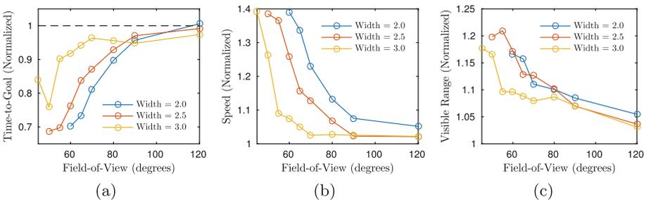
**Fig. 5.** Simulation results: (a) average time-to-goal (lower is better), (b) average speed (higher is better), and (c) average maximum visible range. Averaged results are normalized by the corresponding performance of the baseline planner in the same environments. Plot color indicates hallway width.
