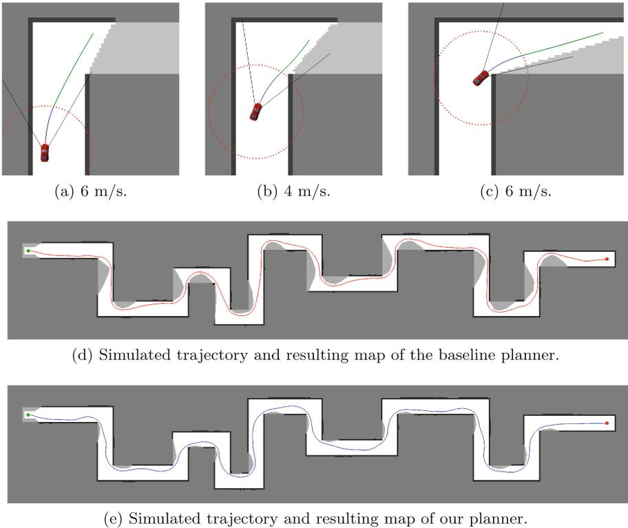
**Fig. 6.** (a)–(c) Example planning sequence using our method, which guides the robot wide around the corner, gaining visibility and maintaining a higher speed. (d)–(e) Simulated trajectory and resulting observed map of the baseline planner and our method, in a 2.5 m hallway with a  $60^\circ$  sensor field-of-view. Green and red dots indicate start and goal, respectively. Dark gray indicates the hidden map, and light gray regions are those that have not been observed.
