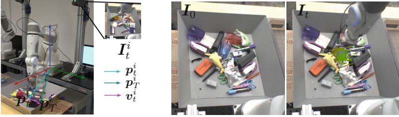
Fig. 2. Left: diagram of the grasp sample setup. Each grasp i consists of T time steps, with each time step corresponding to an image \mathbf{I}_t^i and pose \mathbf{p}_t^i . The final dataset contains samples (\mathbf{I}_t^i, \mathbf{p}_T^i - \mathbf{p}_t^i, \ell_i) that consist of the image, a vector from the current pose to the final pose, and the grasp success label. Right: example input image pair provided to the network, overlaid with lines to indicate sampled target grasp positions. Colors indicate their probabilities of success: green is 1.0 and red is 0.0. The grasp positions are projected onto the image using a known calibration only for visualization. The network does not receive the projections of these poses onto the image, only offsets from the current gripper position in the frame of the robot.
