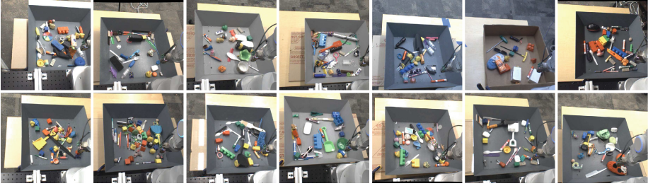
Fig. 4. Images from the cameras of each of the robots during training, with each robot holding the same joint configuration. Note the variation in the bin location, the difference in lighting conditions, the difference in pose of the camera relative to the robot, and the variety of training objects.
