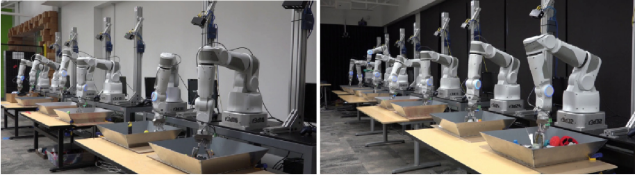
Fig. 1. Our large-scale data collection setup, consisting of 14 robotic manipulators. We collected over 800,000 grasp attempts to train the CNN grasp prediction model.
