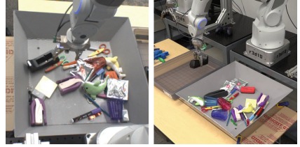
Fig. 5. Previously unseen objects used for testing (left) and the setup for grasping without replacement (right). The test set included heavy, light, flat, large, small, and translucent objects.
