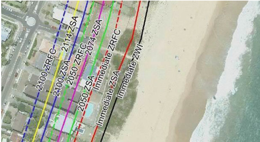
Fig. 21.2 Nine hazard lines reflecting different modelling assumptions and different timeframes for consideration (Source Horton and Britton 2015)
