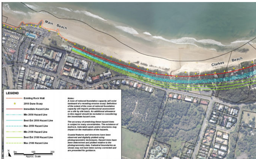
Fig. 21.9 Interpretive descriptors for hazard lines to aid in end use for planning (Source BMT WBM 2013)
