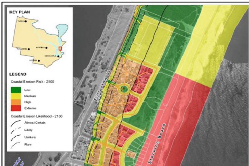
Fig. 21.8 Risk mapping based on spatially represented likelihood and consequence (for 2100) (Source BMT WBM 2014b)
