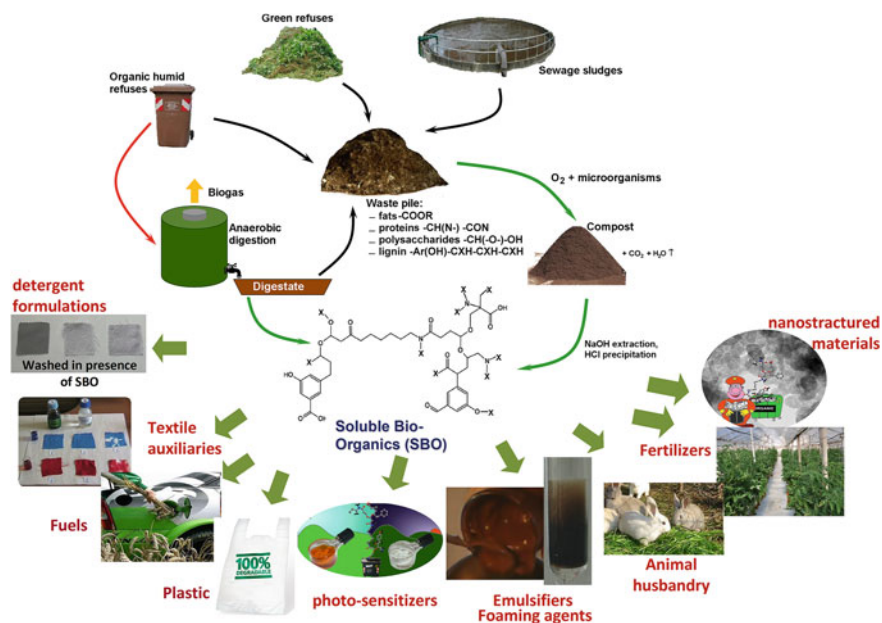
Fig. 6.6 Schematic representation of the sourcing urban bio-wastes, materials obtained by anaerobic and aerobic digestions, and virtual molecular fragment and application fields of soluble bio-based substances obtained by chemical processing of digestate and compost materials by hydrolysis
