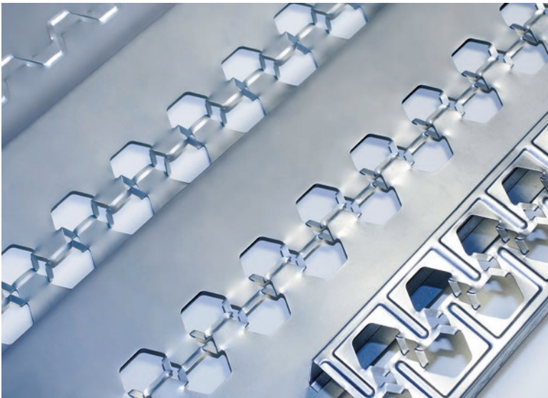
Fig. 24.4 Sheets are cut ( left ), pulled apart ( centre ) and then brought into their final form ( right ) (Source: Protektorwerk Florenz Maisch GmbH)
