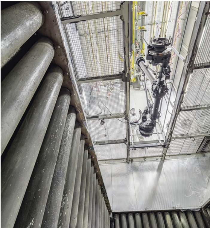
Fig. 24.6 View from the dry separation with the fins ( bottom ) in the painting booth (Source: Daimler AG)
