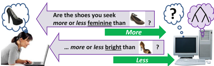
Fig. 5.3 The active version of WhittleSearch requests feedback in the form of visual attribute comparisons between the user’s target and images selected by the system. To formulate the optimal questions, it unifies an entropy reduction criterion with binary search trees in attribute space. Image reprinted with permission
