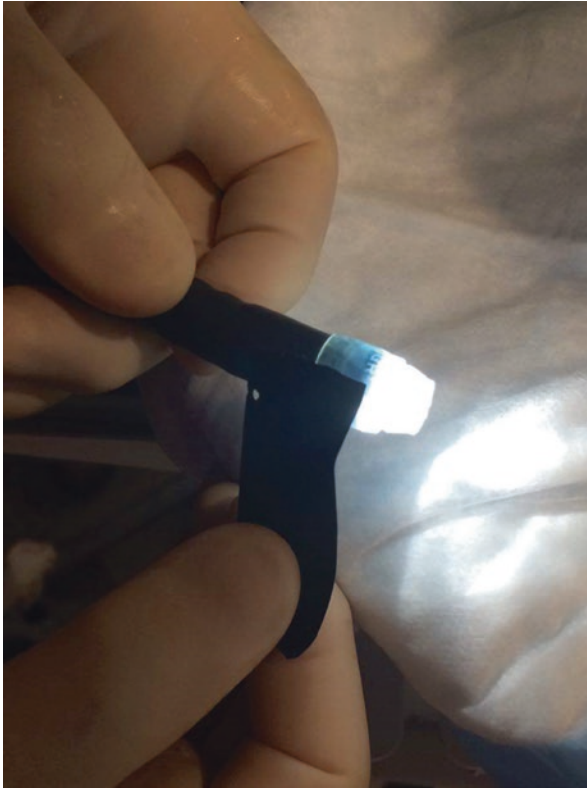
Fig. 3.13 Standard electrical tape to secure the cap to the end of the endoscope
