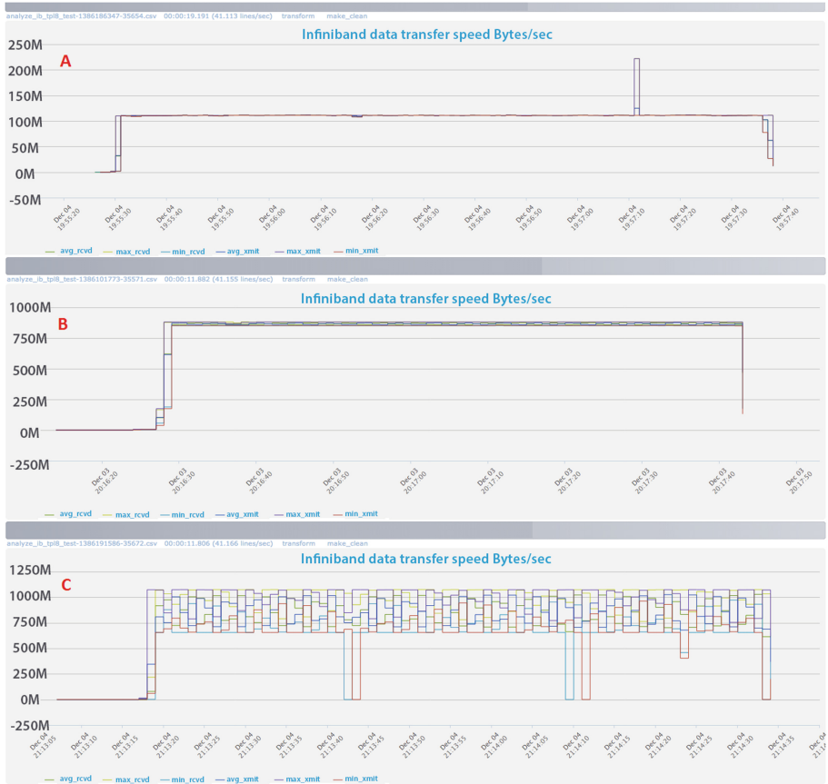
Fig. 2. Data transfer rate over an Infiniband network (A — length 1; B — length 1,000,000; C — length 100,000,000).
