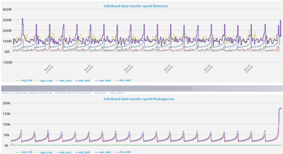
Fig. 4. Data transfer rate over an Infiniband network in MB/sec and packets/sec.
