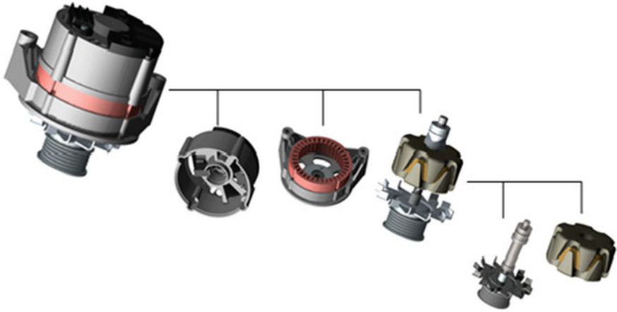
Fig. 9.8 Structured as-designed model of car alternator
