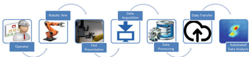
Fig. 12.1 An automated pulsed thermography inspection system
