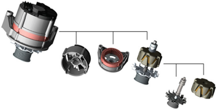
Fig. 9.8 Structured as-designed model of car alternator
