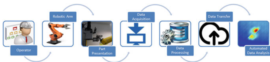
Fig. 12.1 An automated pulsed thermography inspection system
