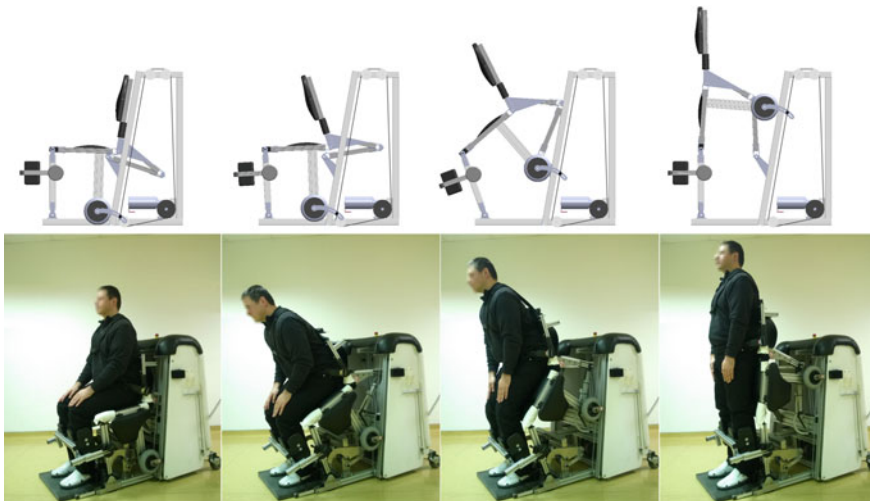
Fig. 5.7 The upper panel shows illustrations of the conceived mechanism while the lower panel shows photographs of the device and neurologically intact subject in four discrete postures during standing-up
