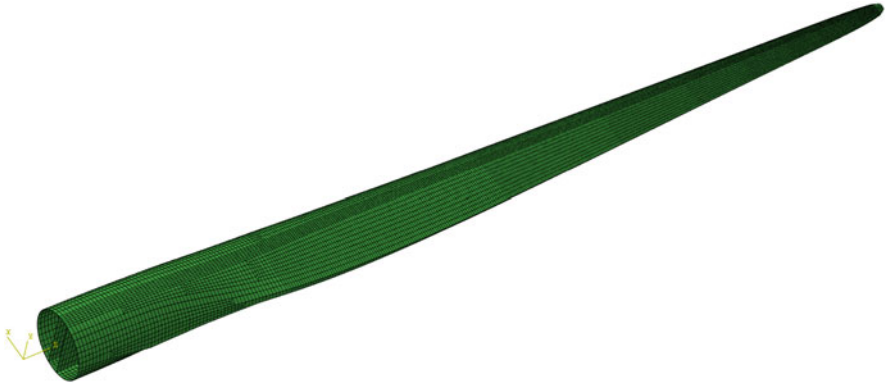
Fig. 6.29 Numerical model of a wind turbine rotor blade
