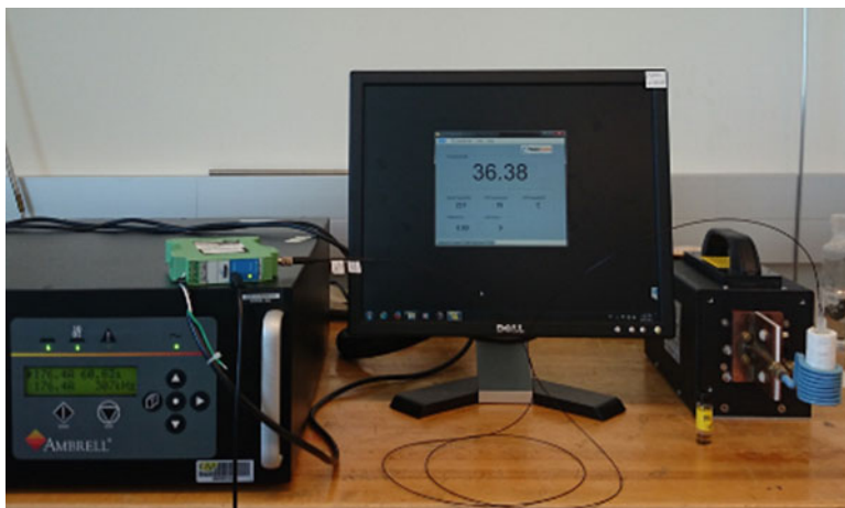
Fig. 7.2 Magnetic hyperthermia system employed. Generator on the left and radio frequency amplifier on the right
