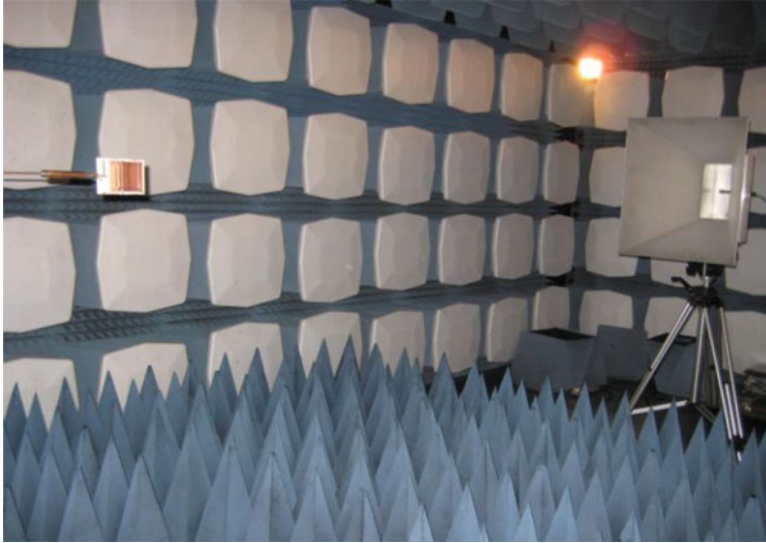
Fig. 9.16 Radiation pattern measurement setup ©Springer [19]
