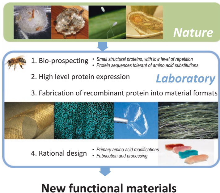
Fig. 15.5 The process used in our laboratory to generate new functional materials. Initially, proteins suitable for high level protein expression and with amino acid sequence that are tolerant of substitutions are identified from nature. The proteins are produced recombinantly and assessed for their ability to be fabricated into material forms. Proteins that fulfil these criteria are then rationally designed to add function
