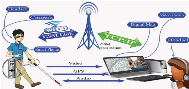
Fig. 1. Tele-guidance system concept
