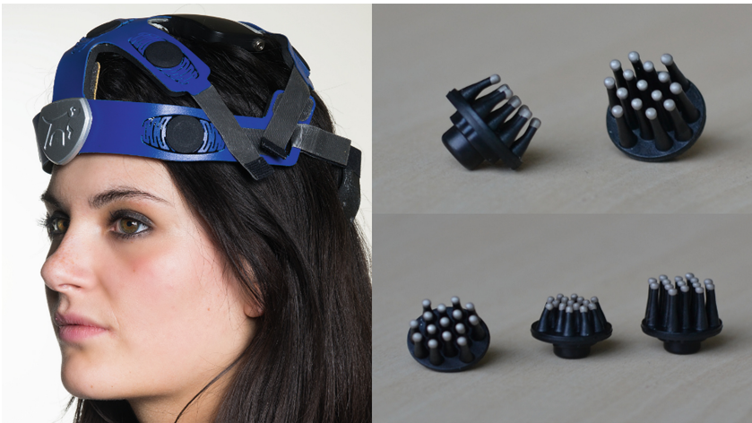
Fig. 1. EEG headset designed by IMEC for cognition monitoring studies. Figures on the right show the polymer electrodes with silver/silver-chloride coating used for data acquisition.
