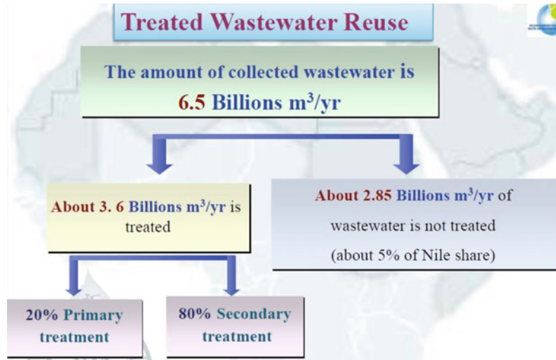
Fig. 14.4 Wastewater supply and treated wastewater for agroforestry (2010). Source HCWW (2011) “Achieving the MDGs for Water and Sanitation Sector in Egypt”
