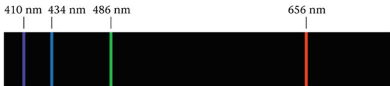
Fig. 5 Emission spectrum of atomic hydrogen in the visible range
