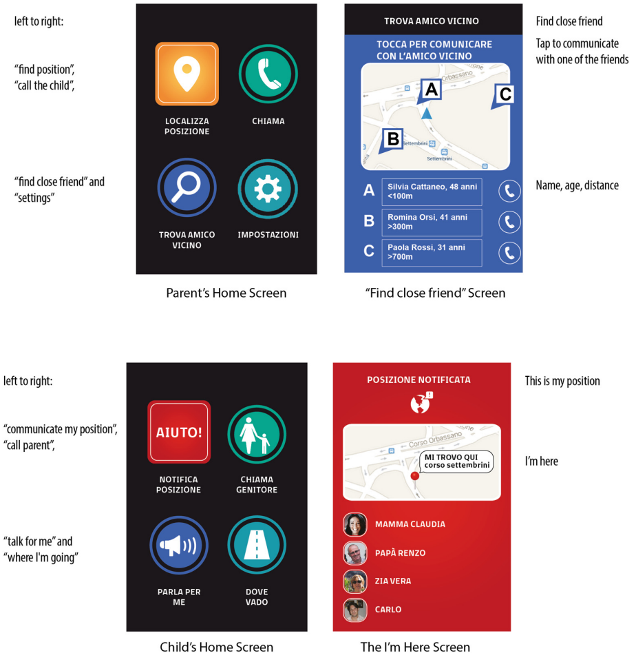
Fig. 2. Examples of the new designed screen's app for the child and the parent [24].
