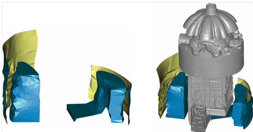
Fig. 9.6 Left 3D visualization of the prospection findings. Right The scanned 3D model (gray) integrated with the 3D GPR data
