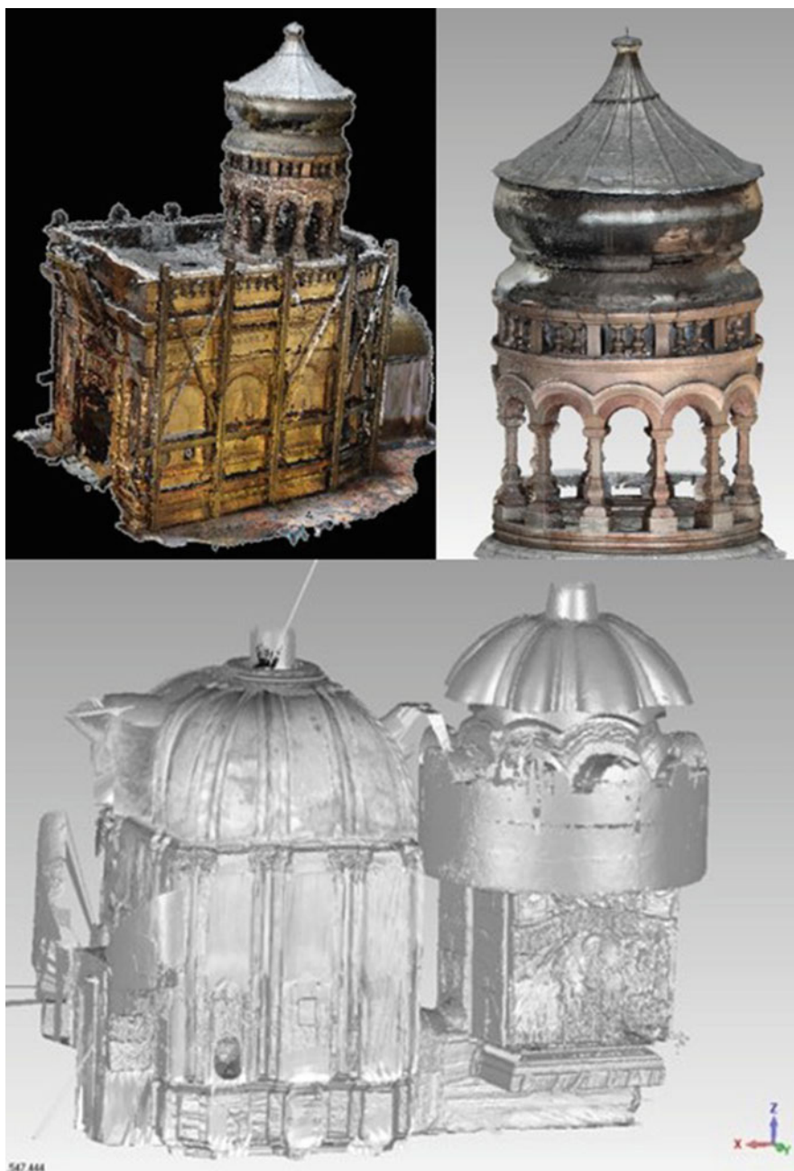
Fig. 9.4 Upper left The colored point cloud of the Holy Aedicule. Upper right The 3D model of the dome textured. Lower Part of the registered point clouds inside the Holy Aedicule [5]
