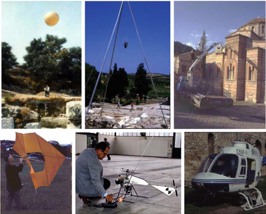
Fig. 2.8 Platforms for aerial photography
