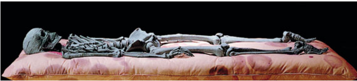
Fig. 21.6 Complete human skeleton. 3D printing (inkjet powder-binder process) (Source: CP-GmbH)
