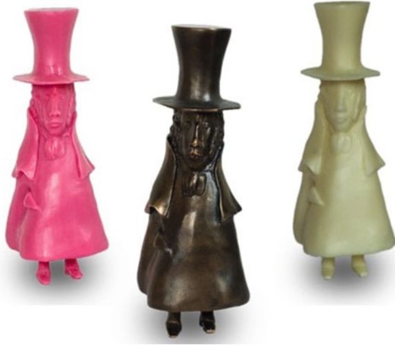
Fig. 21.8 Artistic sculpture by Alisa Minyukova, NY ( white, right ) and RTV copy made from wax ( red, left ) used as a lost wax casting model. Castings made from brass ( center ) (Source: CP-GmbH)
