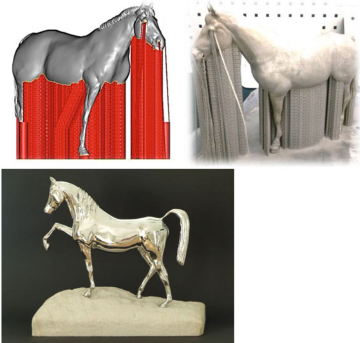
Fig. 21.12 CHIO trophy “Altis MidMesh”. Stainless steel. Print data with supports ( red ) prepared for printing ( above, left ), SLM model with supports after the build ( above, right ), final sculpture (Source: Otto Junker GmbH, GoetheLab FH Aachen)
