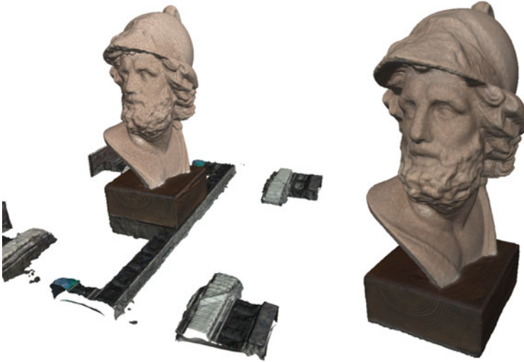
Fig. 4.7 Left to right : color-corrected 3D preview model to identify remaining holes and occlusions; final reconstruction based on consolidated input images from CultArc3D and CultArm3D . © Fraunhofer IGD, Germany, 2016, reprinted with permission
