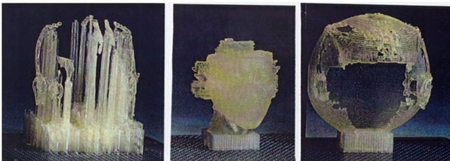
Fig. 21.17 Bust of queen Tiye. Main elements made by AM: Jewelry (on top of the supports), face, bonnet. Stereolithography. Scale: 2:1 (Source: CP-GmbH © 2009, CP GmbH, Germany, reprinted with permission)
