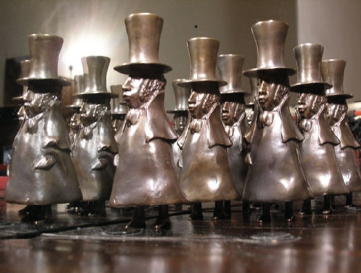
Fig. 21.26 Small series of sculptures made from brass by additive manufacturing and lost wax casting (Source: GoetheLab FH Aachen © 2012 GoetheLab FH Aachen, reprinted with permission)
