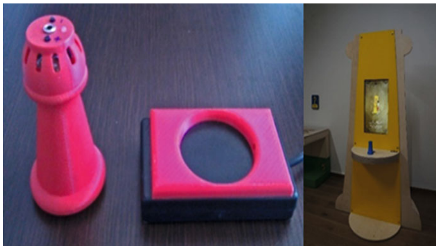
Fig. 19.17 InfoScope device and PC docking station “House of El. Venizelos at the city of Chania” (© 2015 FORTH-ICS, reprinted with permission)
