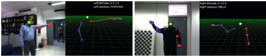
Fig. 18.14 Recognition of pointing ( left ) and waving ( right ) gestures, based on the classification of arm trajectories (© 2010 Sigalas, reprinted with permission)
