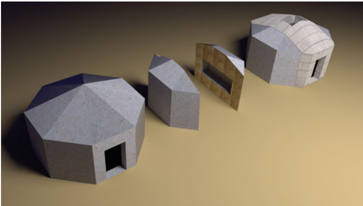
Fig. 9.13 The Holy Aedicule—two construction phases ( left and right models) and the demolished state in the middle
