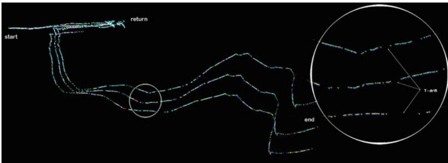
Fig. 3.11 Default motion tracking or pose detection using a generalized camera model, based on feature correspondences. Given three different random seed initializations, the ambiguity is substantial (© 2016 EC FP7 ROVINA project, reprinted with permission)
