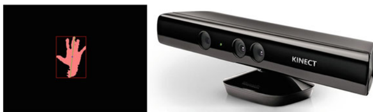
Fig. 16.23 Tracked hand. The position of the centre of the hand is determined in real time by a Microsoft Kinect v1 that provides depth information (MIRALab) (© 2015 Microsoft and Uni. Geneva/MIRALab, reprinted with permission)
