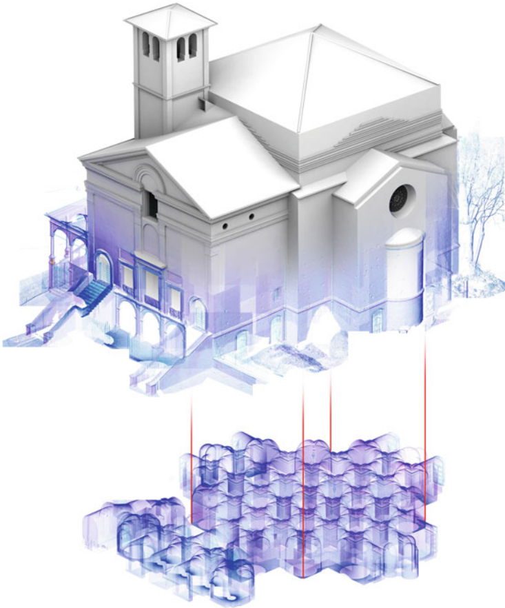
Fig. 8.8 San Sebastiano, Mantua. Hybrid visualization of point cloud and meshed model towards the H-BIM (© 2015 DIAPReM centre, reprinted with permission)
