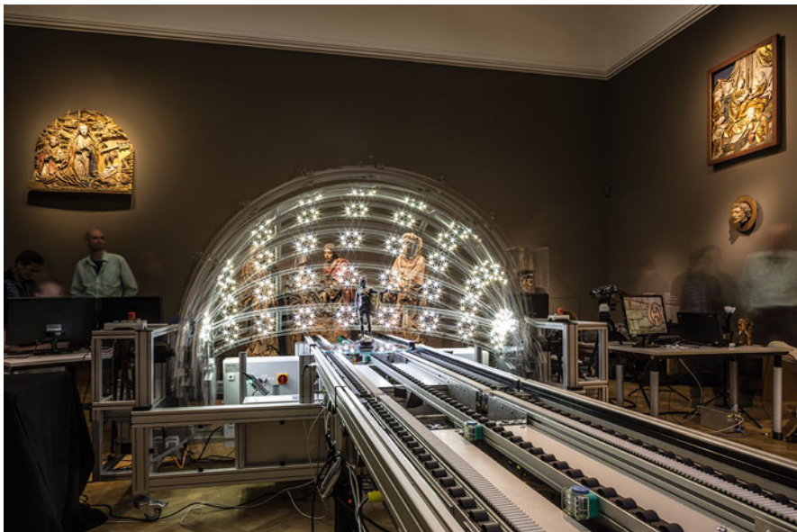
Fig. 4.1 CultArc3D: Two hemispherical rotating arcs, one equipped with cameras, one with ring light sources. Norbert Miguletz © 2014, Liebieghaus Skulpturensammlung, reprinted with permission
