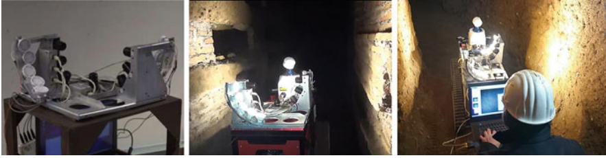
Fig. 3.4 Left : final design of the camera and light arc, here shown on a test trolley. Middle and right : robot carrying camera and light arcs in operation. Note illumination stripe projected on the walls (© 2016 EC FP7 ROVINA project, reprinted with permission)
