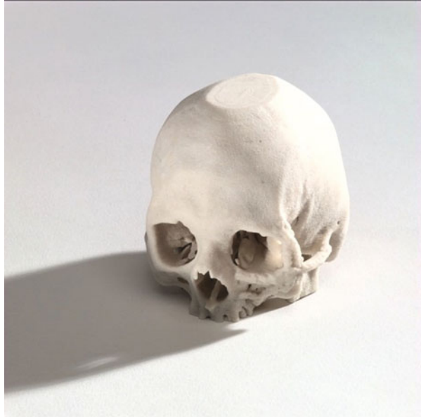
Fig. 21.3 3D printed skull. Inkjet printing (powder-binder process) (Source: 3D Systems/Z-Corp)
