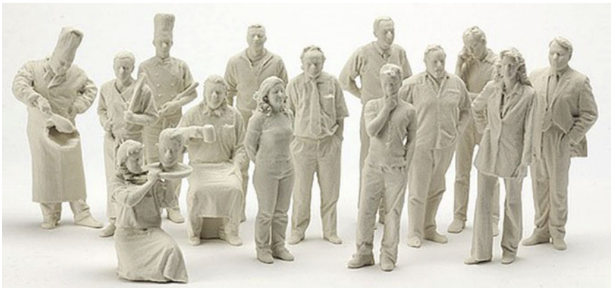
Fig. 21.11 Body scanning and 3D printing (3D Systems/Z-Corp). Plaster-ceramics (Source: Karin Sander/GoetheLab FH-Aachen)
