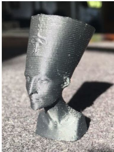
Fig. 21.23 Scaled bust of queen Nefertiti, FDM (ABS), height ca. 5 cm (Source: GoetheLab, FH Aachen © 2012 GoetheLab, FH Aachen, reprinted with permission)
