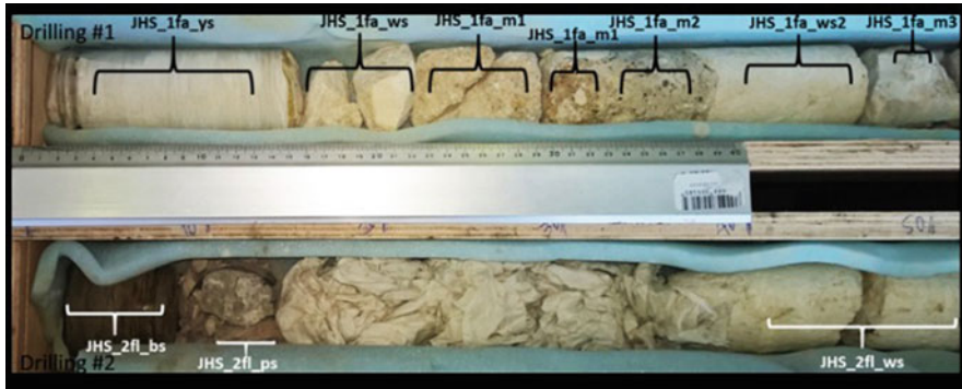
Fig. 9.9 Upper Façade core sample: Three building stones and three mortar samples. Lower Floor core sample: Three building stone samples
