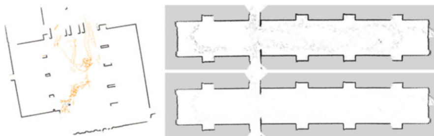
Fig. 18.6 Map of the populated exhibition hall of the Byzantine and Christian Museum in Athens with measurements labeled as belonging to dynamic objects shown in orange ( left ). Maps created for the populated corridor environment of the University of Bonn without and with people filtering ( right ) (reproduced from [27], © 2003 by Taylor & Francis, reprinted with permission)
