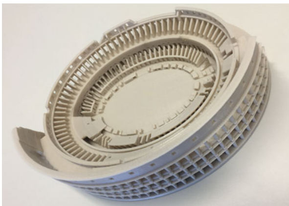
Fig. 21.7 Reproduction of the Roman Colosseum. Plastic filament printer (Source: Data Thingiverse; Print, GoetheLab, FH Aachen)
