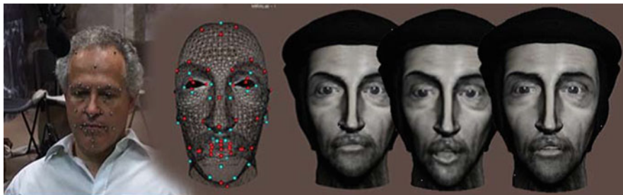
Fig. 16.13 From motion capture to 3D facial animation—Calvin facial animation (MIRALab) (© 2008 Uni. Geneva/MIRALab, reprinted with permission)
