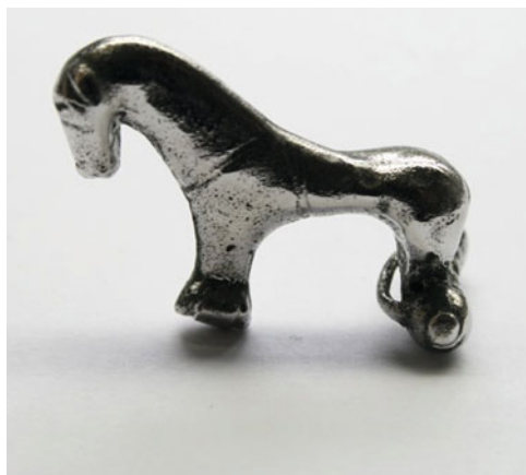
Fig. 21.25 Celtic garment pin (fibula). Scanned and made from metal by SLM (Source: GoetheLab FH Aachen © 2013 GoetheLab FH Aachen, reprinted with permission)
