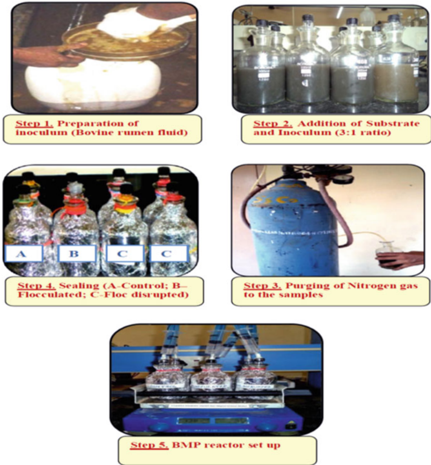
Fig. 2 Experimental set-up of BMP assay
