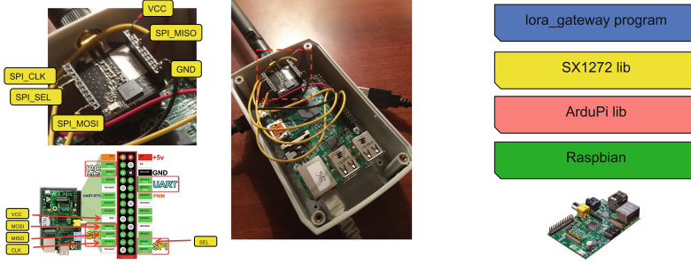
Fig. 3. Low cost gateway from off-the-shelves components
