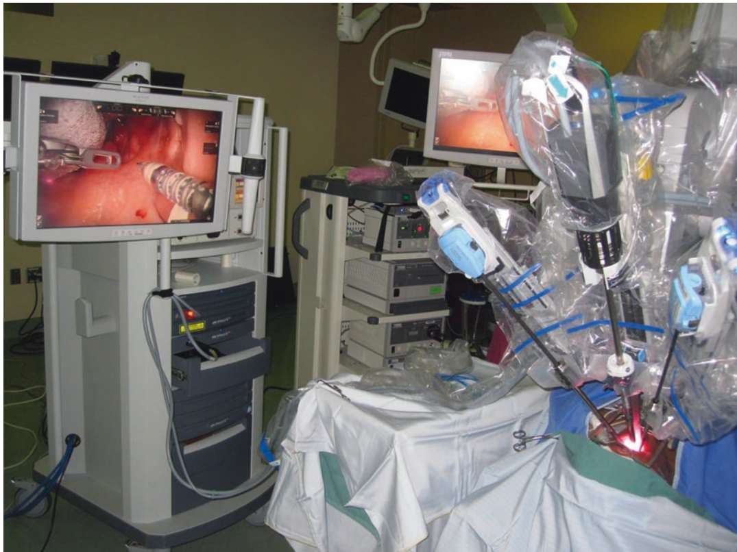
Fig. 2.4 Example of da Vinci robotic arm orientation and vision cart placement. Note central camera, ipsilateral monopolar cautery, and contralateral forceps placement
