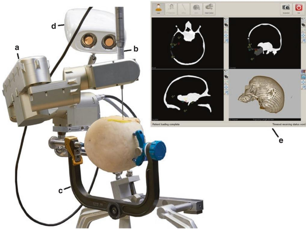
**Fig. 17.6** Overview of the robot navigation system. (a) The mounted robot to the OR table, (b) a conventional surgical drill, (c) a head clamp, (d) an optical tracking system, and (e) a touch screen interface [17]
