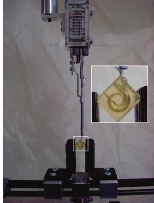
**Fig. 17.5** Experimental setup of electrode insertion above the scala tympani model [26]
